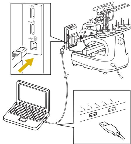
If the machine is positioned at a distance that prevents the USB cable from reaching the computer, embroidery patterns can be transferred from the computer by temporarily saving them on USB media or an SD card, which is then inserted into the machine. (Refer to “Saving embroidery patterns to USB media/SD card” on page 160.)
