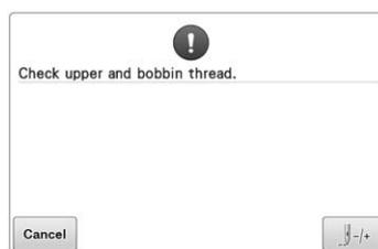
**The upper thread broke, the thread came out of the thread tension disc or a thread guide, or the machine is not threaded correctly.**
