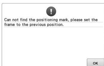
**When embroidering the pattern for the optional jumbo frame, the machine failed to find the positioning mark.**
