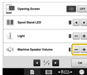
→ Check that the desired speaker volume is selected with the operation sound produced when a key is touched.
