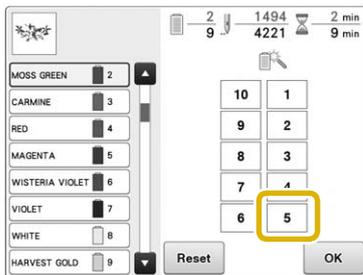
→ The needle bar number changes and
