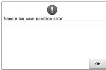
**The needle bar case has stopped at an incorrect position.**
