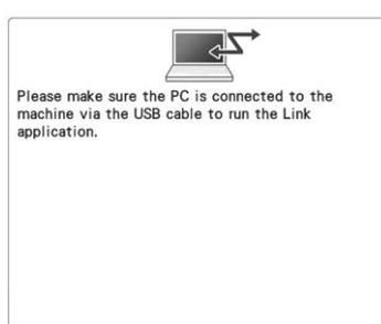
Machine failed to communicate with the PC in the Link mode.
