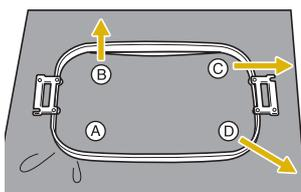
First, align the inner and outer frames at the corner with the screw (A). Then, while lightly pulling the fabric in the direction indicated by arrow (B) so that the fabric is taut, insert the inner frame at corner (B). In the same way, lightly pull the fabric in the direction indicated by arrow (C) and insert corner (C), and then lightly pull the fabric in the direction indicated by arrow (D) and insert corner (D).
