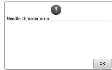
**The automatic needle-threading mechanism did not operate correctly.**
