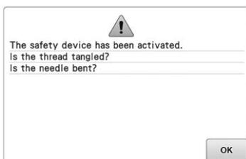
**The motor has locked up due to tangled thread or for other reasons related to thread delivery.**
