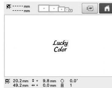
When the key displayed as
