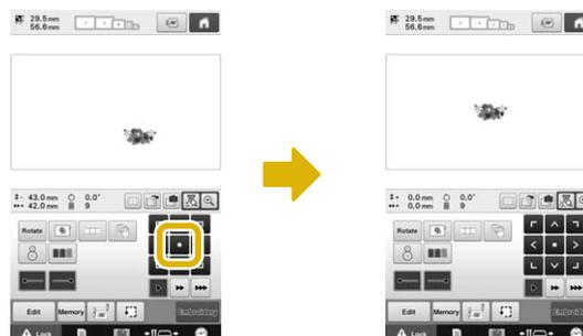
The pattern can also be moved by dragging it. If a USB mouse is connected, move the mouse to position the pointer on the desired pattern, and then while holding in the left mouse button, drag the pattern. The pattern can also be dragged by selecting it directly in the screen with your finger or the touch pen.
