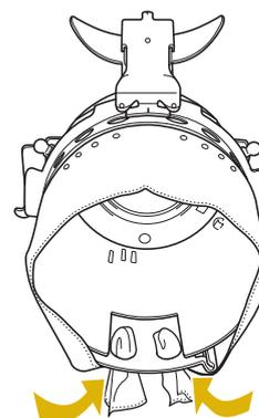
**6** Lift out the sweat guard on the inside of the cap, and then place the cap over the cap frame.
