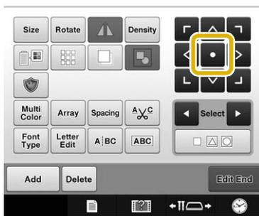
The pattern can also be moved by dragging it. If a USB mouse is connected, move the mouse to position the pointer on the desired pattern, and then hold in the left mouse button while dragging the pattern. The pattern can also be dragged by selecting it directly in the screen with your finger or the touch pen.
