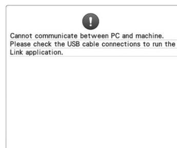
**Machine cannot receive any data from the PC in the Link mode.**
