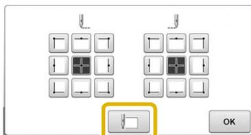
→ The needle bar is positioned in the lower-left corner of the pattern. The embroidery frame moves so that the needle is positioned correctly.
