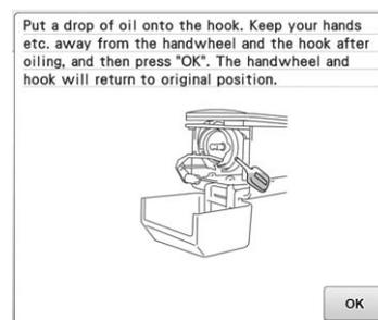
7 After oiling, insert the bobbin case into the hook, and then close the hook cover. (Refer to page 37.)
