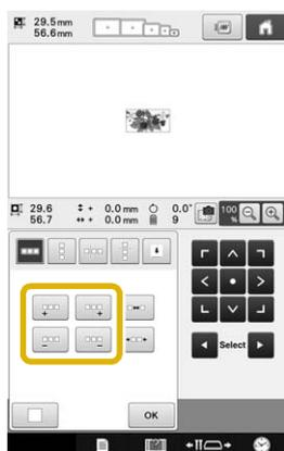
**4** Adjust the spacing of the repeated pattern.
