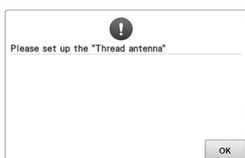
Thread guide assembly support is not prepared.
