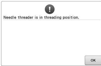
**Another operation was performed while the automatic needle-threading mechanism was threading the needle.**
