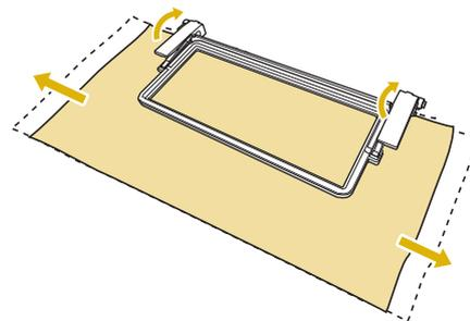
**1 Create the repeated pattern with the thread mark at the center of the end of the pattern.**
