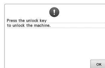
The thread trimming button was pressed before the machine was unlocked.
