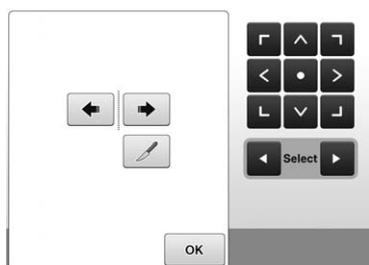
**2 Use** **to select where the pattern is to be separated, and then touch** **to separate it. For this example, the pattern will be separated between “T” and “a”.**
