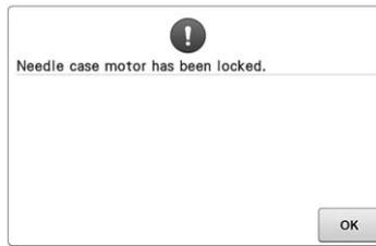
**The needle bar case motor has locked up.**
