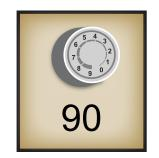
2. Adjust the tension by turning the tension dial clockwise to tighten and counter-clockwise to loosen. The tension value appears on the touch screen. The value changes as you turn the tension dial.
