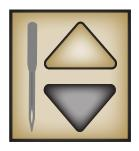
**Needle-stop button:** Touch the button to alternate between having the needle stop in the up or down position when you press the stop/start button to stop stitching. Your choice displays in gold.
