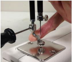
NOTE: Before threading the needle, test that the machine is threaded properly and the tension is correct by carefully pulling the top thread. It should pull smoothly with light to medium tension. If thread pulls freely with no tension, re-thread the machine, ensuring that the thread is flossed into the tension discs.
