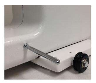
3. Slide the laser clamp onto the mounting post and tighten the two knobs on opposite sides of the clamp.
