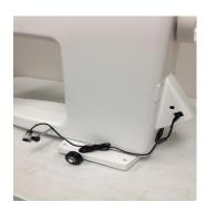
4. Plug the laser cable end into the laser stylus port on the back of the machine. This is found on the tension side of the machine inset in the rectangular shaped opening.
