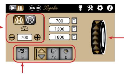
The on-screen hand wheel enables you to rotate the machine's hand wheel from the main screen rather than reaching around the machine to do it manually.
