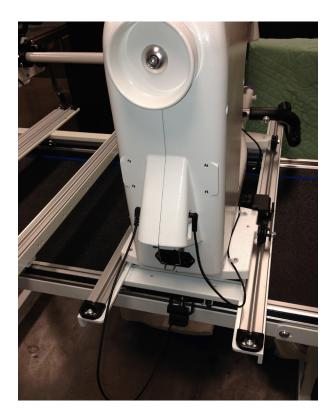
**■ IMPORTANT**: If you ever need to remove the machine from the carriage, disconnect the stitch regulator cable from the machine. Failure to unplug the cable when removing the machine from the carriage could result in damage to the cable, encoders, and carriage.
