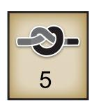
Tie-off button: Use this button to perform a tie-off at the start or finish of your stitching. Touch the button and gently move the machine to perform the micro stitches. The number below the image indicates how many micro stitches will
