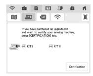
• Press App Guide in the settings screen or machine help screen to view details on the two apps available through the upgrade kits. In order to use the app, the corresponding KIT must be certified.
