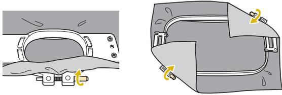
**5** Securely tighten the screw, and then check to make sure that the fabric is taut.
