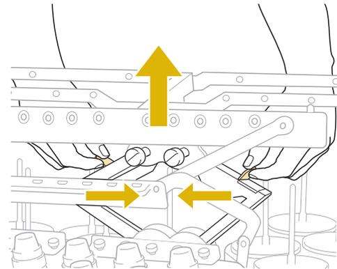
**3 After the thread guide assembly support is extended and the thread guide assembly is raised to its highest position, tighten the two thumb screws to secure the thread guide assembly in place.**
