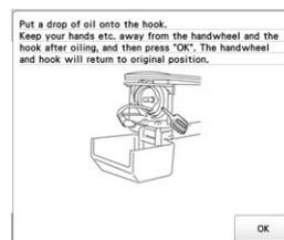
7 After oiling, insert the bobbin case into the hook, and then close the hook cover. (page 35)
