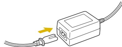
**2** Plug the cord on the AC adapter into the DC input connector of the bobbin winder, and then insert the plug of the power supply cord into a household electrical outlet.
