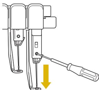
→ The needle and presser foot are locked in the down position.
