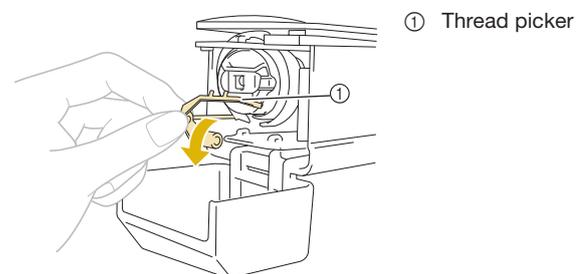
To gain access to the bobbin case easily, pull the thread picker toward front.
