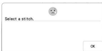
This message is displayed when there is no stitch pattern selected and the "Start/Stop" button or the "Reverse/Reinforcement Stitch" button is pressed.
