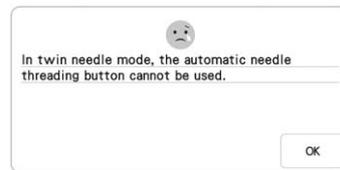
This message is displayed when the automatic needle threading button is pushed while twin needle sewing is set.
