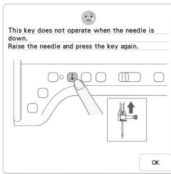
This message is displayed when a key on the LCD display is touched while the needle is in the down position.
