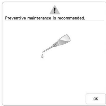
Once this message appears, it is recommended to take your machine to an authorized Baby Lock retailer for a regular maintenance check. Although this message will disappear and the machine will continue to function once you press , the message will display several more times until the appropriate maintenance is performed.
