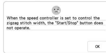
This message is displayed when the speed control lever is set to control the zigzag stitch width, and the “Start/ Stop” button is pushed. Use the foot controller to operate the machine.
