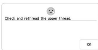
This message is displayed when the upper thread is broken or not threaded correctly, and the "Start/Stop" button or the "Reverse/ Reinforcement Stitch" button is pressed.
