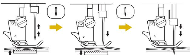
\* When the needle is nearly lowered by pressing the "Needle Position" button, the feed dogs are lowered. At this time, the fabric can be shifted to finely adjust the needle drop position.
