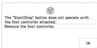
This message is displayed when the "Start/Stop" button is pushed to sew utility stitches or character/ decorative stitches while the foot controller is connected.
