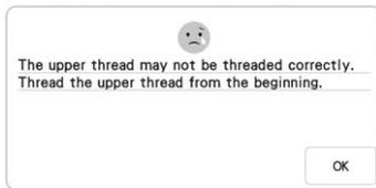
This message is displayed when it seems that the upper thread has not been threaded correctly.
