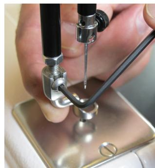
4. Ensure the middle of the foot opening is centered with the needle when the foot is fully tightened with the 2.5mm hex wrench. If it isn't properly centered, loosen the lock nut on the foot adaptor with an 8mm wrench, center the foot with the needle; hold the foot firmly in position; and tighten the lock nut.
