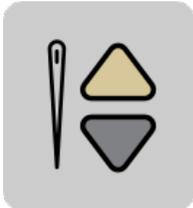
**Needle-stop button:** Touch the button to alternate between having the needle stop in the up or down position. When the stop/start button is selected to stop stitching, the needle-stop position is gold.
