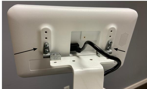
3. Plug the USB mini B cable (with 90° connection), coming out of the top front cover, into the back of the display. This cable provides power and signal connection from the machine to the display.
